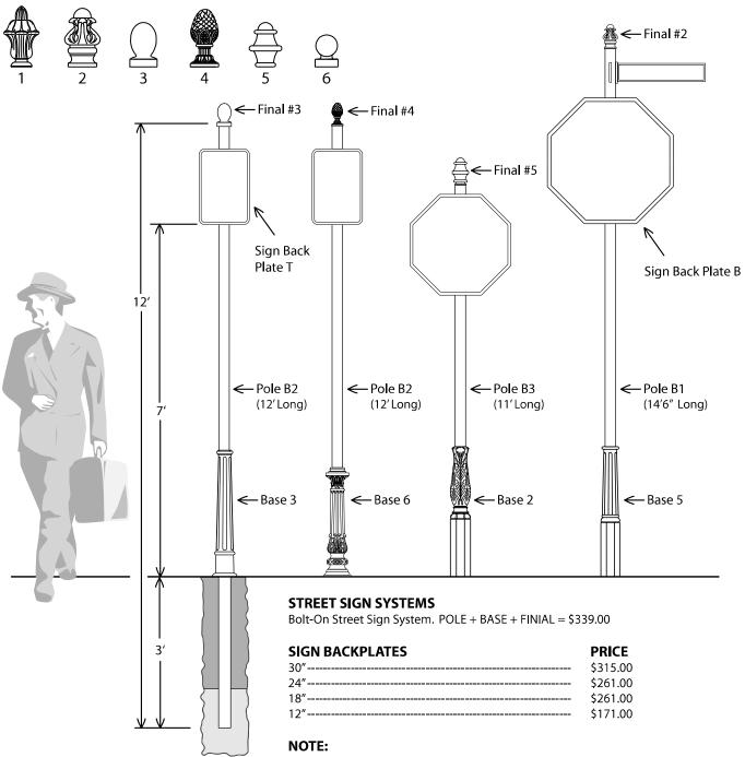
The "B" post is a 2 3/8" round post and is either 11',12', or 14.5' long. The "Sign Back Plates" are nice, but for a more economical solution, see our "pip post mounting brackets" at....
